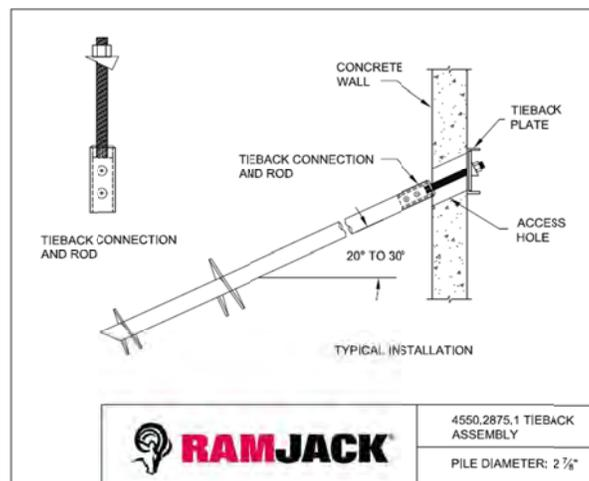
FIGURE 10—4550.2875.1 TIEBACK ASSEMBLY
