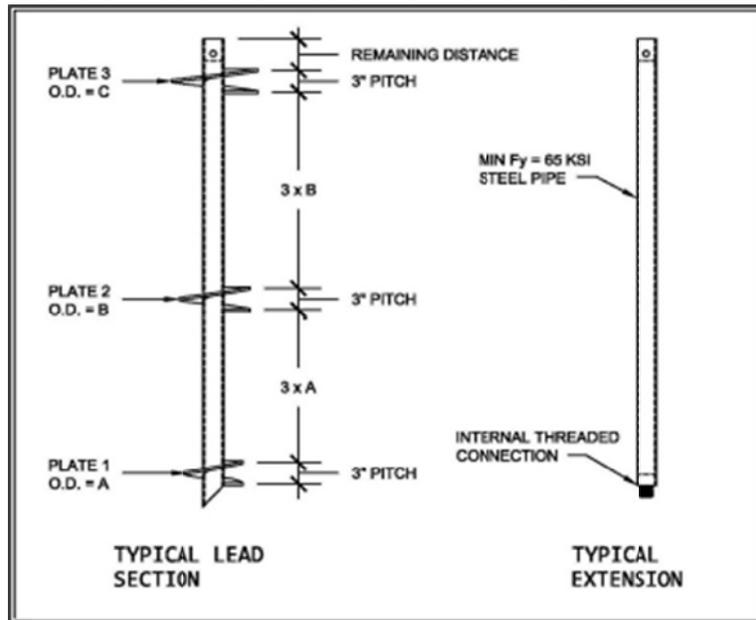
FIGURE 1—TYPICAL HELICAL PILE AND PLATE SPACING CHARACTERISTICS
